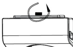
2. Allow the tank to stand in the correct position, and open the tank cover by turning anti-clockwise.
