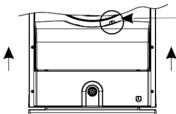
1. Remove the screw with a screwdriver, and lift the water tank at both sides keeping it level.
