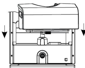
4. Turn the tank upside down and re-install it on the fan.
