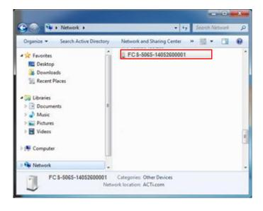
By double-clicking with the left mouse on the camera model, it is possible to automatically launch the default browser of the PC with the IP address of the target camera filled in the address bar of the browser already.
