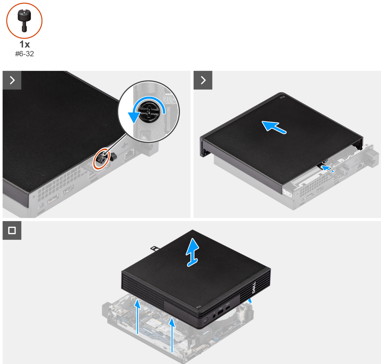
Figure 10. Removing the side cover
