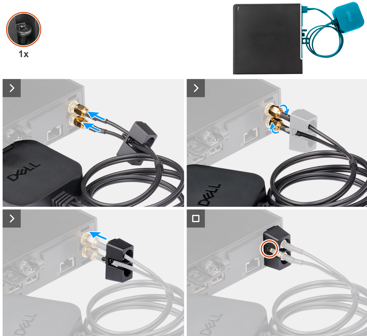
Figure 35. Installing external puck antenna
