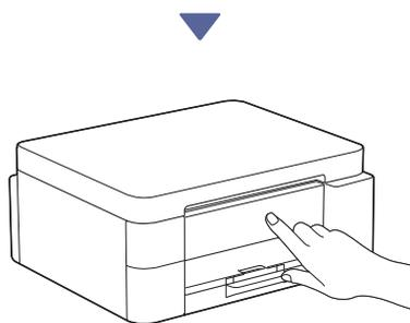
Check the LCD messages to continue the setup. When the ink preparation message appears, follow the LCD instructions to perform the initial ink system cleaning. Cleaning can take a few minutes, and you can perform the next step during this time.
