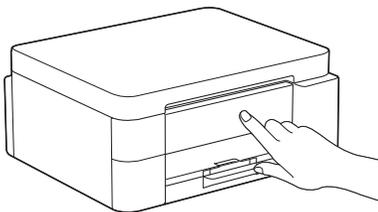
On the machine's LCD, select the images that closely match the image for each colour on the Print Quality Check Sheet, and then restart the cleaning procedure, if required.
