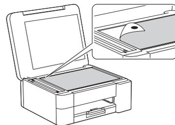
Place the Adjustment Sheet face down on the scanner glass, making sure the black circle is in the top left corner of the scanner glass, as shown.
