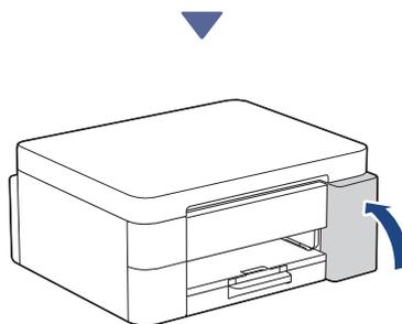
After installing all of the four ink cartridges, close the ink cartridge cover.
