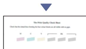
When the initial ink system cleaning has finished, the machine prints the Print Quality Check Sheet.
