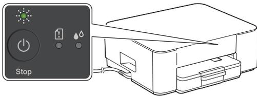
The machine powers on automatically and the Power LED starts flashing.
