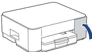
After installing all of the four ink cartridges, close the ink cartridge cover. The machine will start the initial ink system cleaning.
