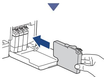
Install the inbox ink cartridges.
