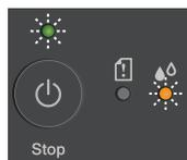
During the initial cleaning, both the Power and Ink LEDs will flash.
