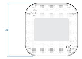
The illustration shows the height and width dimensions of the chassis. Dimensions are in millimeters. The chassis width is 130mm (side to side). The height from the bottom of the system to the top of the system including the rubber feet is 34mm.
