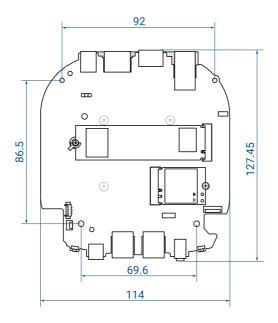
The illustration shows the height dimensions of the board. Dimensions are in millimeters. The tallest feature on the user accessible side of the board when in use is the M.2 retention feature, and on the CPU side is the thermal module.
