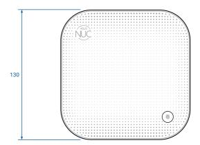
The illustration shows the height and width dimensions of the chassis. Dimensions are in millimeters. The chassis width is 130mm (side to side). The height from the bottom of the system to the top of the system including the rubber feet is 34mm.
