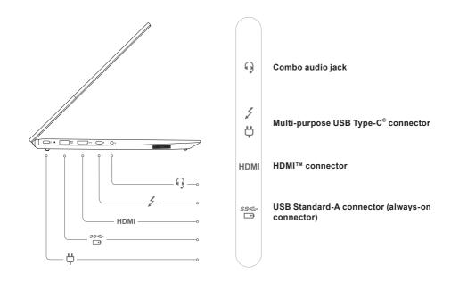
👔 The USB Type-C connector with an icon 🌶 is Thunderbolt 🕮 4 enabled. The USB Type-C connector with a plug icon 🛱 next to it also functions as the PC's power input connector.
