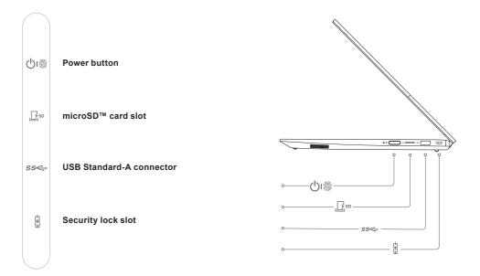
i The power button includes an embedded fingerprint sensor.
