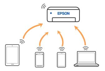
The printer can be connected by Wi-Fi or Ethernet, and Wi-Fi Direct (Simple AP) connection simultaneously. However, if you start a network connection in Wi-Fi Direct (Simple AP) connection when the printer is connected by Wi-Fi, the Wi-Fi is temporarily disconnected.
