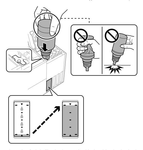
9. When you have finished refilling the ink, remove the ink bottle, and then close the ink tank cap securely.
