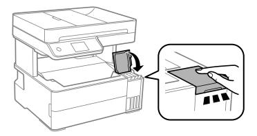
11. Insert the accessory box that came with the printer with the opening flap facing forward as shown below.
