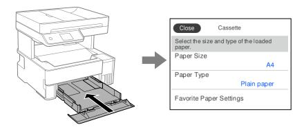
If displayed paper size and type differ from the loaded paper, select the item to change. If the settings match the loaded paper, close the screen.
