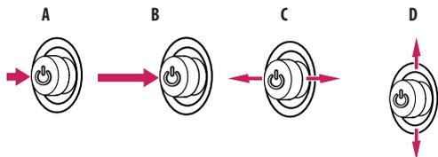
**A (Power on):** Press the joystick button once with your finger to turn on the monitor.
