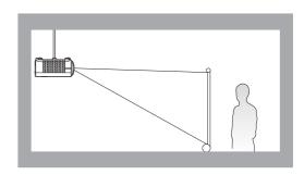
After turning on the projector, the projector will automatically select a suitable setting for the way the projector is installed. If not, go to the **Advanced** Menu - **Installation** > **Projector Position** and press **◄**/**▶** to select a setting.
