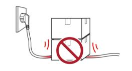
If the product emits a strange sound, burning smell, or smoke, turn off the power immediately and unplug the power cord. If the product is dropped or its exterior is damaged, turn off the power immediately and unplug the power cord. Do not subject the product to shock. It may start a fire. It may damage the product.
