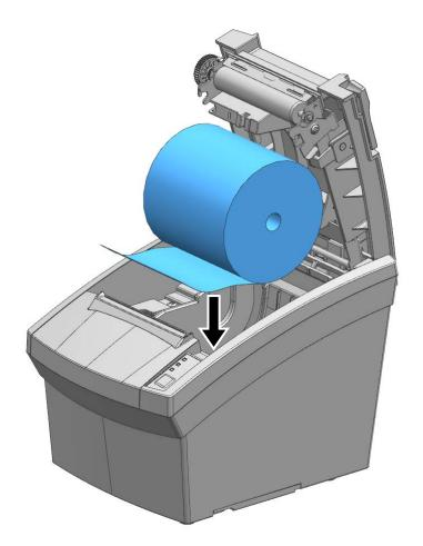
3) Check the orientation of the roll paper when inserting it into the printer.
