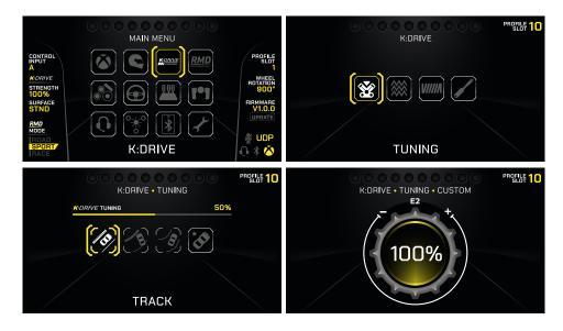
The **K:DRIVE** section allows you to tune multiple aspects of the Direct Drive motor. This feature is per-profile, so different force feedback responses can be saved and accessed on-the-fly.
