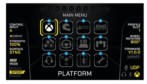
The **MAIN MENU** contains all the different options for configuring the VelocityOne Race. Rotate the **E2 dial** to show the menu and cycle through the different options. Press the **Select button** to enter the option or press the **Back button** to return to the Dashboard. All the customization options you can adjust are stored in the onboard memory. These are divided into two types:
