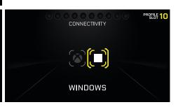
The **PLATFORM** section allows you to change the input mode of the product. It will be in Xbox mode by default. Rotate the **E2 dial** to highlight the platform icon and press the **Select button** to activate. The system will reboot to be used on the platform and the input mode will be stored in memory for next time you use the wheel.
