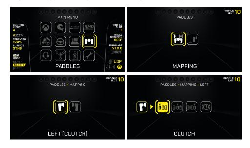
The **PADDLES** section allows you to alter the response characteristics of the analogue paddles located below the gear shifters. This feature is per-profile, so different responses can be saved and accessed on-the-fly.
