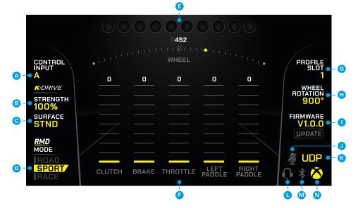
The **DASHBOARD** serves as the home screen of the Race Management Display (RMD). It displays the current state of the system, including active profile slot, K:Drive motor settings, RMD output settings, Wheel Rotation and connectivity status. It also shows the real time input of all the axes and buttons on the product.
