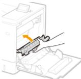
2 Lower the green levers on both sides of the transport guide.
