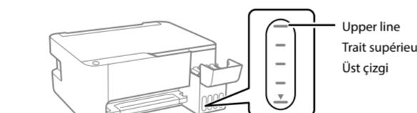
Insert the ink bottle straight into the port to fill ink to the upper line.
