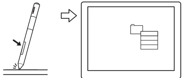
PAN/SCROLL lets you position a document or image in any direction within the active window simply by pressing the pen button and moving the pen tip across the tablet. As you move the pen tip, the document or image is repositioned to follow the direction of pen movement on the tablet. Release the pen button or lift the pen tip from the tablet surface when done.
