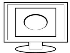
When FORCE PROPORTIONS is checked, the correct vertical and horizontal proportions are maintained. Drawing a circle on the tablet results in a circle on the display screen. Depending on your settings, some portions of the tablet active area may no longer be usable when this option is selected.
