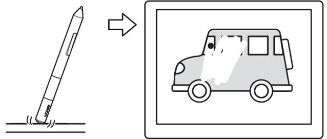
Use the pen eraser in Windows 8, Windows 7, and Vista to erase notes or sketches made with [Pen and digital ink capabilities in Windows](#), and to select and delete text or spreadsheet cells within an application. In supporting text applications use the eraser to select text, then lift the eraser from the tablet to delete the text.
