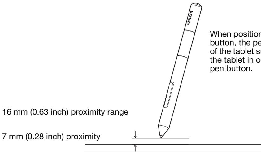
When positioning the screen cursor and operating a pen button, the pen tip needs to be within 7 mm (0.28 inch) of the tablet surface. The pen tip does not need to touch the tablet in order to move the screen cursor or use a pen button.
