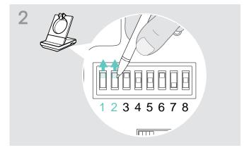
> Use a pointed object to set the DIP switches 1 and 2 to the position shown.
