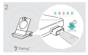
Press and hold the dongle's button for 3 seconds to enter pairing mode.
