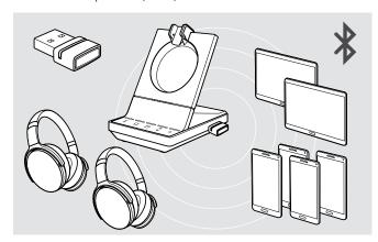
The dongle can save up to eight paired Bluetooth devices. If you pair a ninth device, the saved connection profile of the least used Bluetooth device will be overwritten.
