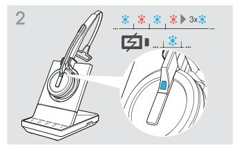
If the headset and base station are not paired, the headset LED flashes blue and red shortly. The LED turns blue when pairing is complete and the headset will start charging.
