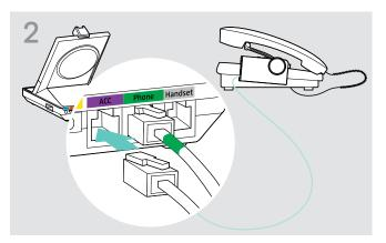
> Connect the handset lifter to the ACC socket on the base station.
