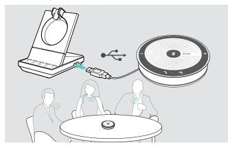
To use an external speaker with microphone such as the EPOS speakerphone SP 20:
