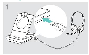
Connect the headset to the USB socket on the base station.
