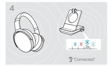
Once the Bluetooth devices are paired, the LED flashes 3 times blue and then lights up in a constant dim blue.
