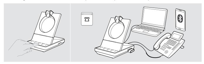
> Touch the icon of the desired audio source on your base station  $\Box/\Box/\Box$ . The chosen audio source is in focus and the LED lights up white.
