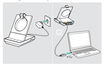
> Disconnect the base station from the mains power supply and the computer.
