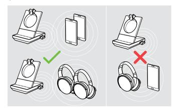
After switch-on, the dongle automatically tries to connect to the two last connected Bluetooth devices - mobile phone and headset cannot be combined.
