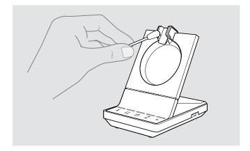
> Clean the charging contacts of the base station and the headset from time to time using e.g. a cotton swab.
