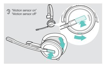
> Press the volume button as shown and simultaneously the hook button. Hold the buttons until you hear three beeps.
