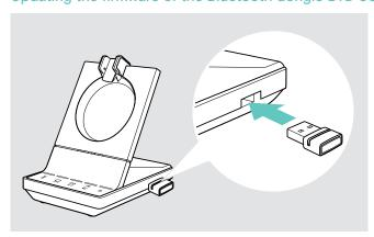
Insert the BTD 800 into the USB port on the base station. Some older dongle versions need to be connected directly to the computer in order to be updated. "New" dongles can be identified by the two grey lines on the bottom side of the housing.
