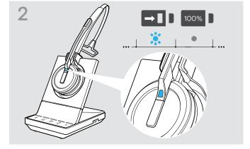
> Place the headset into the magnetic holder of the base station. The headset battery status LEDs on the base station indicate the charge status.
