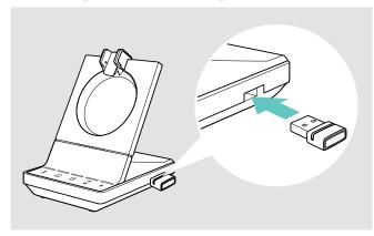
The BTD 800 dongle is supplied together with the SDW 50X4 and SDW 50X6 bundles and also available as an accessory.
