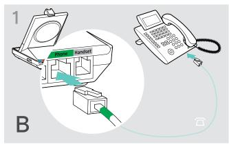
> Connect the telephone cable to the headset socket on the telephone and to the Phone socket (marked green) on the base station.
