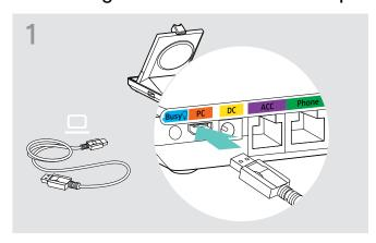
> Connect the USB cable to the PC socket on the base station.
