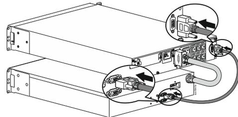
**NOTE:** Secure the communication cable to the UPS and the XLBP. The UPS will display inaccurate runtime if the connection is not secure.
