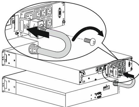
**NOTE:** Be sure secure the battery connector with the supplied pan head screw.
