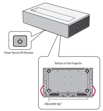
1) Turn the adjustable leg left or right to adjust the angle.
