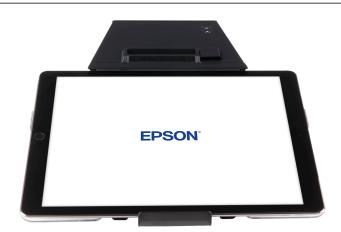
The TM-m30II-SL is an all-in-one POS solution that's comprised of the TM-m30II and a tablet stand in one stylish, space-saving unit.
