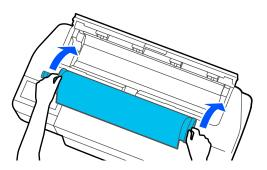
Check that the leading edge of the roll paper is not bent and then insert it into the paper slot until you hear a beep.
