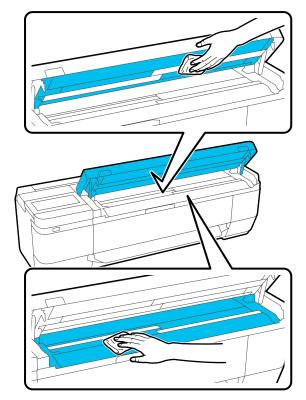
Use the cleaning kit, or the clean side of the soft cloth, to thoroughly wipe the area shown in blue in the illustration below.
