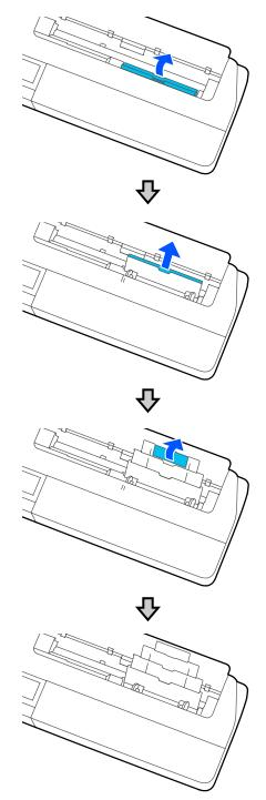
Load paper in the auto sheet feeder with the printable side facing you.
