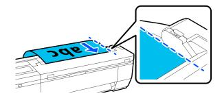
When the leading edge touches the back of the paper slot, the document is automatically fed to the scanning start position. When automatic paper feeding starts, let go of the document and do not interfere with the document feeding operation. When you hear a beep, feeding is complete.
