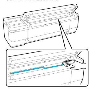
Use the cleaning kit, or the clean side of the soft cloth, to wipe the glass surface.
