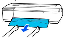
Open the front cover, remove the jammed paper, and then close the front cover.
