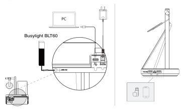
Note: Please make sure you connect the base to a DC power supply, not just the USB power supply. The included USB-A to USB-C cable cannot be used to connect other devices (for example, mobile device) to the USB hub port.
