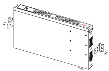
Note: Whenever possible, attach two screws into wall studs. If stud mounting is not possible, use an expandable wall anchor. Hardware is not included; 25" x 2" lag bolts are recommended. Mount the UPS in either of the displayed positions.
