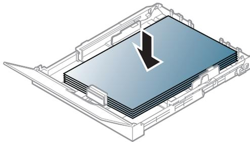
For paper smaller than A4-sized, press and unlatch the guide lock in the tray, push the tray in manually. Then adjust the paper length guide and paper width guide.
