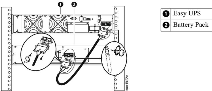
1. Locate the battery connector cover on rear panel of UPS and battery pack.
