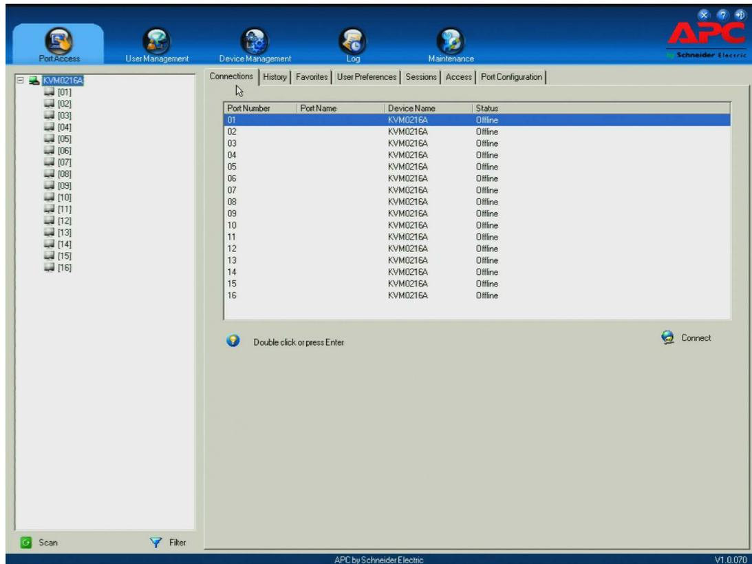
The Connections page is organized into several main areas. All the devices, ports, and outlets that a user is permitted to access are listed in the Sidebar at the left of the page.
