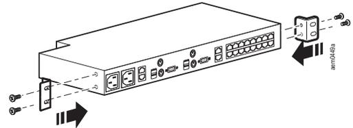
2. Install the smaller bracket from the front of the unit to the back. Install the rack mounting bracket from the inventory to the rear of the unit.
